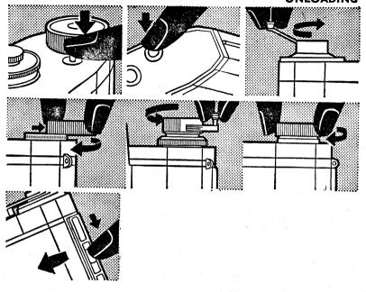
Top, left: Depress rewind button on camera top plate on all models except Prakticamat.
