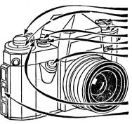
Transport lever Film counter Rewind crank Film speed indicator Slow speed setting Shutter speed dial Flash contacts Shutter release
