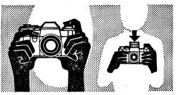
For horizontal shots (above) hold the camera in the palm of both hands, the fingers gripping the front of the body, and the thumbs against the back. Focus the lens with the thumb of the left hand.
