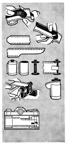
Top: The standard trims of film end and leader with trimming template. The full trim need not be made for the Praktica. A small trim of the leader is, however, necessary to enable it to be inserted in the take-up spool.
