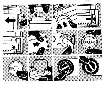
Top, left to right: Open the camera back (I, All Praktica except L range. 2, Opening back of L range); pull up the rewind knob, insert the cassette and push the rewind knob back; attach film to take-up spool, so that it winds emulsion out on all models since Praktica IV. Models from Nova I onward have quick-load take-up spools.
