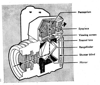
Above: The viewing system of the models from Praktica IV onwards presents a right-way-up, right-way-round image at the viewfinder eyepiece. This sectional view shows the light path through the lens via the angled mirror and the pentaprism to the eyepiece.
